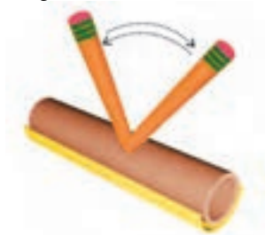
Fig. 5.5 Directions of movement allowed by a hinge like joint
