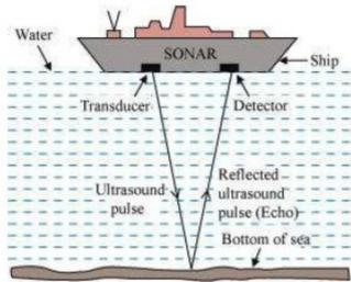
A beam of ultrasonic sound is produced and transmitted by the transducer (it is a device that produces ultrasonic sound) of the SONAR, which travels through sea water. The echo produced by the reflection of this ultrasonic sound is detected and recorded by the detector, which is converted into electrical signals. The distance (d) of the under-water object is calculated from the time (t) taken by the echo to return with speed (v) is given by
