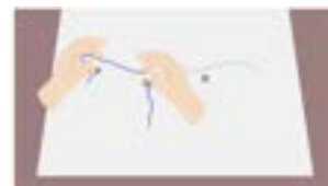
Measuring a Curved Line
