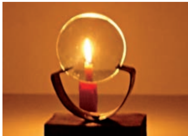
Fig. 11.27 Image formed by a concave lens
