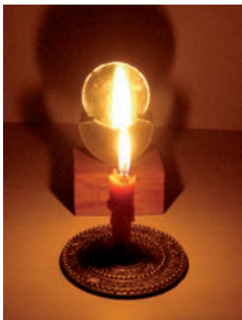
Fig. 11.16 Virtual image formed by a concave mirror
