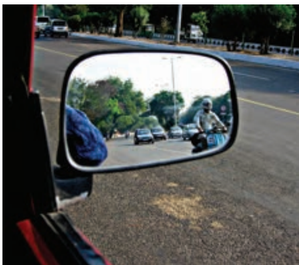
Fig. 11.20 Convex mirror as side view mirror
