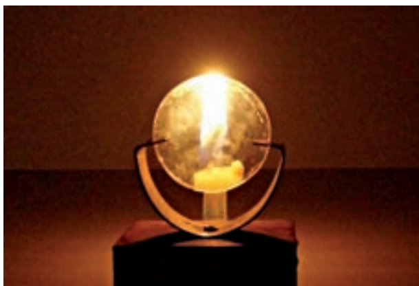
Fig. 11.26 Virtual image formed by the convex lens
