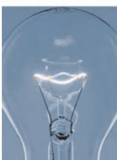
Fig. 10.12 Glowing filament of an electric bulb (incandescent)
