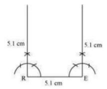
(3) As vertex A and D are 5.1 cm away from vertex E and R respectively, cut line segments EA and RD, each of 5.1 cm from these rays.
