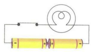
Answer. The bulb in the Circuit iS not glowing because the two cells are not connected properly. To make the bulb glow, the negative terminal of one cell Should be connected to the positive terminal of the other cell, as shown in the given figure.
