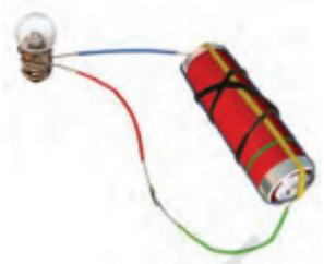
Answer. The bulb will not glow. This is because the two terminals of the cell are connected to the single terminal of the bulb. This is equivalent to the bulb not being connected in the circuit at all. The two terminals of the battery should be connected to the two terminals of the cell.
