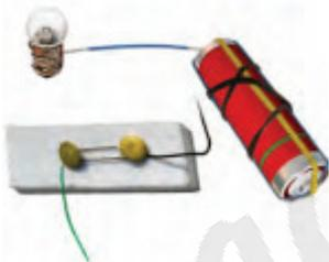
Answer. The given circuit is not complete. To complete the circuit, the positive terminal of the cell should be connected to one end of the switch, and the other terminal of the bulb should be connected to the other end of the switch. The closed circuit is shown in the following figure:
